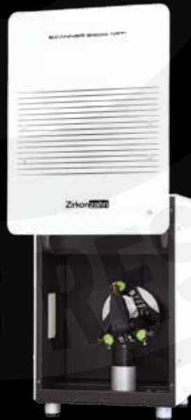
5 S600 ARTI scanner with articulator (Zirkonzahn)
