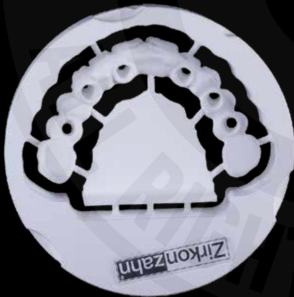
12, 13 The milled structure with connectors and sintering stabiliser
